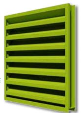
The ELF211D is a 2" deep stationary louver featuring 38% free area with a high performance frame system and a drainable head to help collect and remove water. This louver also has an architecturally styled hidden mullion, allowing a continuous blade appearance.
