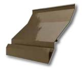
The ELF375DX Stationary Louver has a 4" deep frame, 54% free area, and all aluminum construction for low maintenance and high resistance to corrosion.
