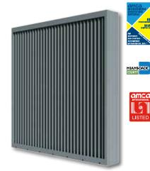
The EME6625D Stationary Rain-Resistant Louver has a 6" deep frame and vertical blades, 43% free area, and excellent pressure drop performance.
