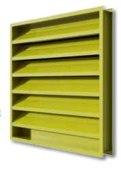
The ELBD812 Combination Louver has a 4" deep frame, operable blades, 40% free area, and constructed for low maintenance and resistance to corrosion.
