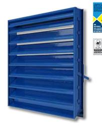
The ELM6DW Adjustable Warehouse Louver has a 6" deep frame, adjustable blades, 48% free area, and is AMCA certified for water penetration & air performance.
