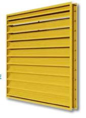
The ELC445D Combination Louver has a 4" deep frame, drainable blades, 39% free area, and aluminum construction for COMBINATION LOUVER low maintenance and high corrosion resistance.
