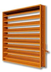
The ELM90 Adjustable Louver has a 6" deep frame, 70° blade angle, 58% free area, and excellent protection against weather exposure.
