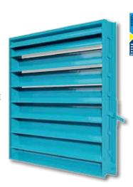
The ELM6375X Non-Drainable Adjustable Louver 371/2° blade angle, 6" frame depth, 54% free area, and low torque.
