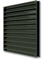
The L45 Steel Non-Drainable Adjustable Louver has a 4" deep frame, 45° blade angle, 38% free area, and tight shut off for excellent weather protection.
