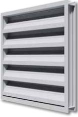
The ELF211D is a 2" deep stationary louver featuring 42% free area with a high performance frame system and a non-drainable head.
