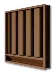
The L5361 Stationary Louver is a 4" deep sand removal louver. It has 27% free area, 90% particle removal efficiency, sight proof blades, and is both AMCA 500-L and ASHRAE Standard 52-76 listed
