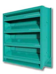
The ELC6375DAX Louver has a 6" deep frame, AMCA listed for 511, 47% free area, and architecturally styled hidden mullions allowing continuous line appearance up to 120".
