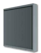
The EME6625 Stationary Rain-Resistant Louver has a 6" deep frame, vertical blades, 43% free area, AMCA 540/550 listed, and excellent pressure drop performance.
